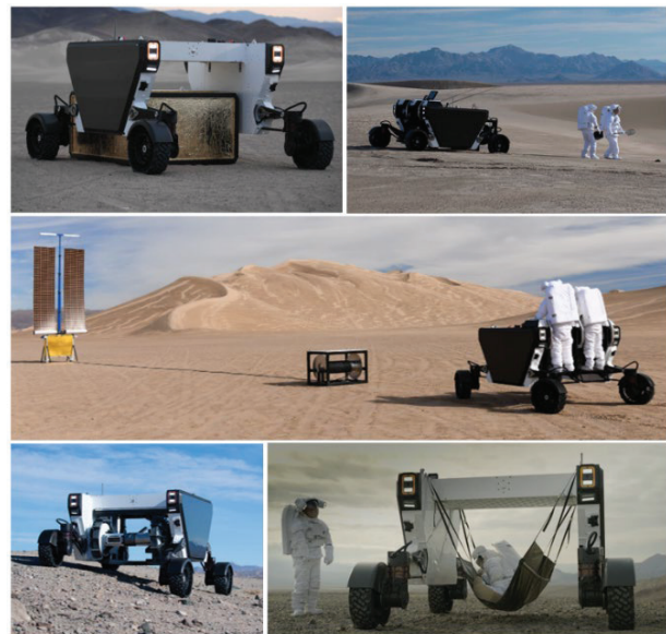
Figure 2: FLEX's modular payload interface and novel mobility system enable it to perform a multitude of functions, including (left to right, top to bottom): outpost logistics, crew exploration and science, infrastructure deployment, robotic science, and crew rescue tasks
