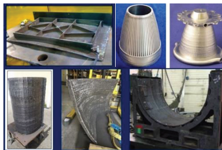
Fig 1. (Top-Left & Bottom) Large metal components manufactured by Keystone using in-house robotic Wire Arc Metal AM cell. (Top-Right) Channel wall nozzle closed out using Laser Wire AM.
