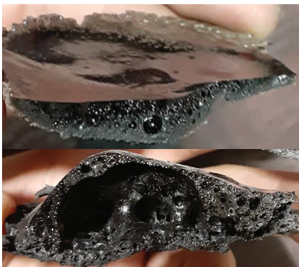
Figure 1: JSC-1A samples after being produced and cooled in open air (Upper) and in vacuum (Lower).
