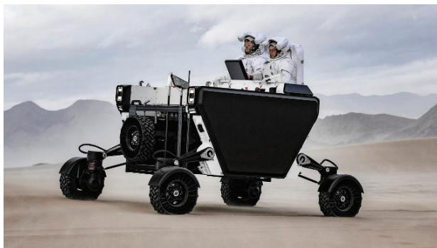
Figure 1: The FLEX rover is an LTV-class mobility platform with adaptive utility enabled by modular payloads
