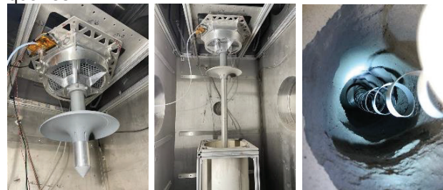
Figure 3: (left) Instrument in stowed configuration (middle) Deployed stated after burial of sonde (right) Sonde deployed at target depth with umbilical ribbon cable.
