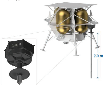
Figure 1: Instrument mounted on the belly-pan of a lander using DIABLO to deploy the sonde up to 2 meters from a stowed configuration.
